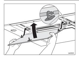
■ To replace a panel, hold it firmly with both hands, hook it over the retaining bar (see detail in the illustration), tilt the panel upwards and press it into the locking clip at the front until you hear it click into position.
